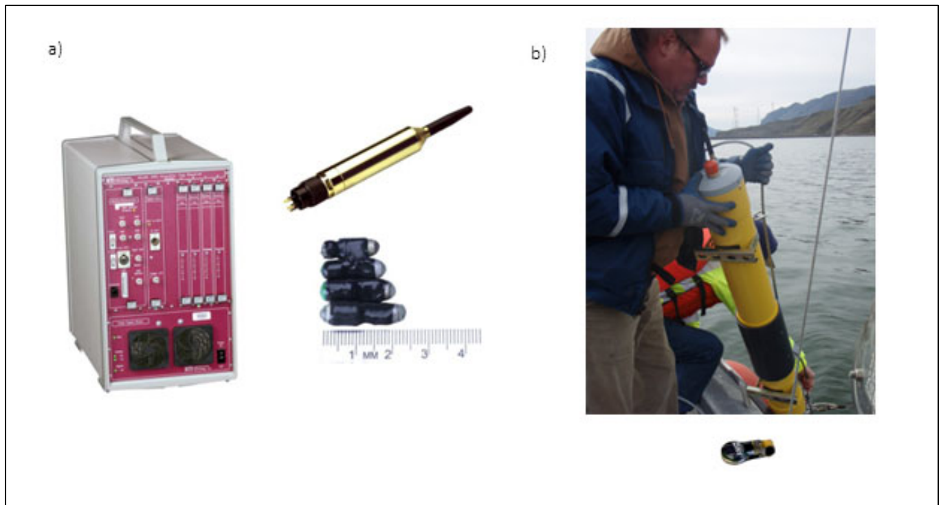
Figure 2. Acoustic technologies used in previous studies: a) HTI 290 receivers with cabled hydrophones and 307 kHz tags; and b) JSATS autonomous acoustic receivers and JSATS and 416 kHz tags.
